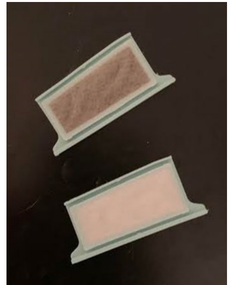
A brand new CPAP filter (bottom) and after four nights of use in “Very Unhealthy” PM 2.5 conditions (top).
